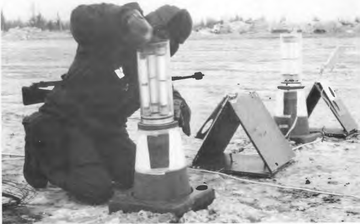
Tritium light developed at the Laboratory is installed at an Alaskan airfield by an Air Force employee.
