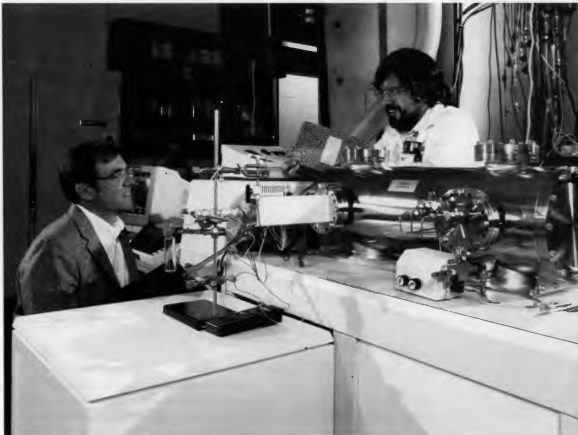
Mike Guerin and Mark Wise work at an ion-trap mass spectrometer used for quickly identifying and quantifying pollutants. A portable version of the ORNL system provides on-site soil, water, and air analyses.
