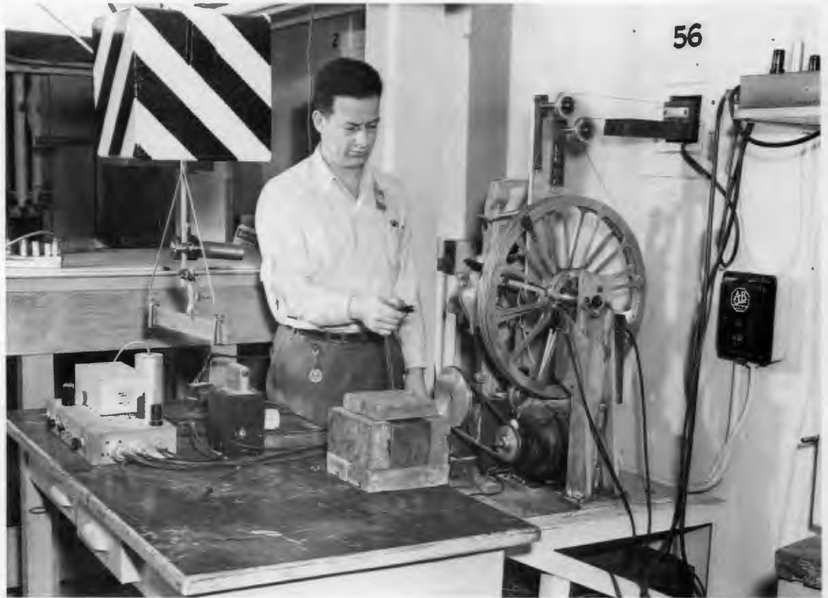
Herbert Pomerance uses a washing-machine mechanism (called the pile oscillator) to oscillate materials in and out of the Graphite Reactor for neutron irradiation.
