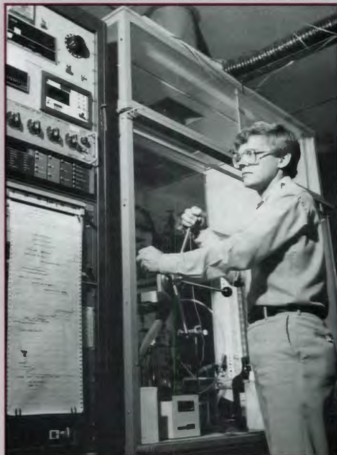
Don Palmer injects a solution into an electrochemical cell in an experiment to determine the nature of a sample of chromium.
