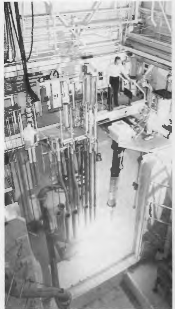
Cerenkov glow of nuclear fission in water was visible at the Bulk Shielding Reactor.
