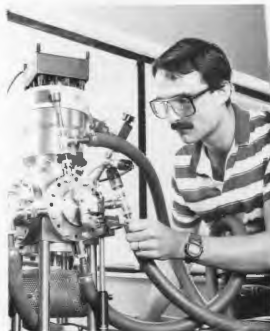
Scott McLuckey adjusts an ion trap for analyzing ionized DNA fragments.
