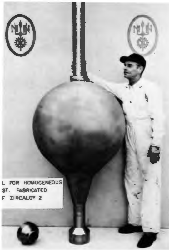
Bulb-shaped core vessel built for ORNL's experimental Homogeneous Reactor Test.
