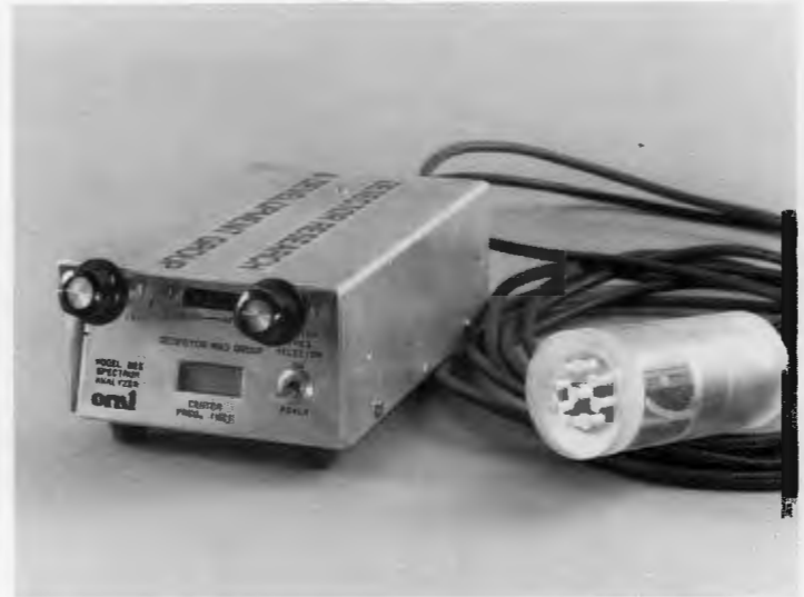
ORNL’s Bee Spectrum Analyzer can detect Africanized killer bees in European honeybee hives.
