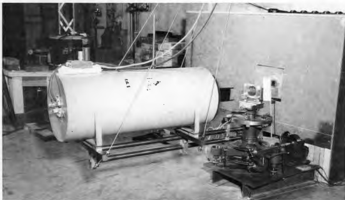
The first two-axis diffractometer for neutron scattering research included an X-ray instrument that Ernest Wollan had used at the University of Chicago before bringing it to the Laboratory. Part of this instrument is displayed at the Smithsonian Institution.
