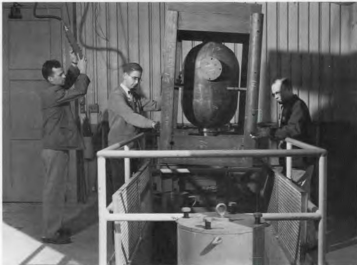
Henry Grimoc, W. R. Casto, and G. L. Neely prepare a container for shipping radioactive cobalt-60 from the Laboratory to Los Angeles for use in treating cancer patients.
