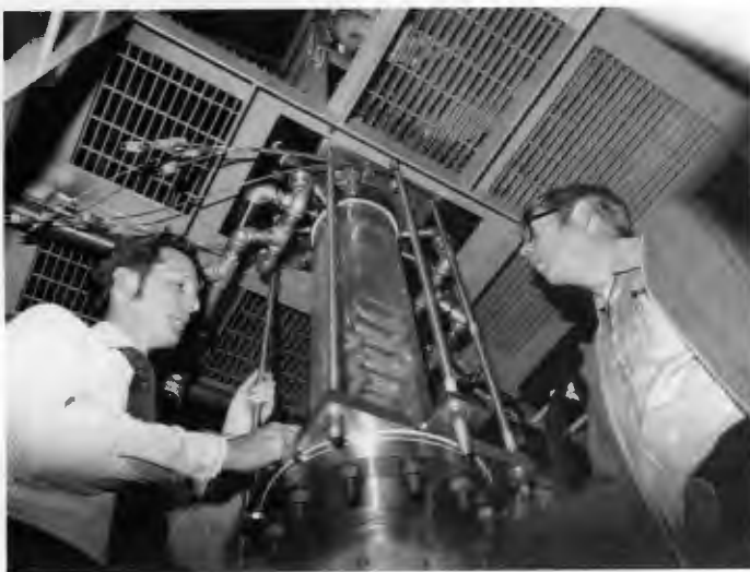
Robert Holcomb and John Jones examine a fluidized bed for coal combustion developed at the Laboratory.
