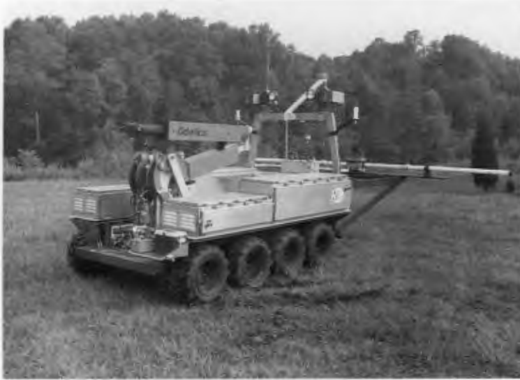
To speed mapping and measurement of contamination, the Laboratory improved a remotely operated vehicle for survey of waste sites.
