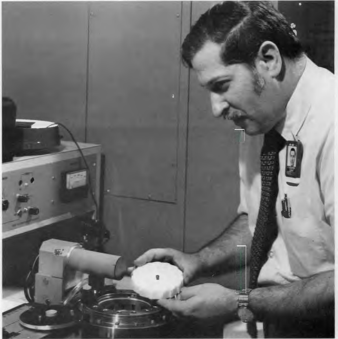
Gerald Goldstein tests the ability of the GeMSAEC analyzer to detect and measure trace pollutants in air and water—one symbol of the Laboratory's scientific diversity.
