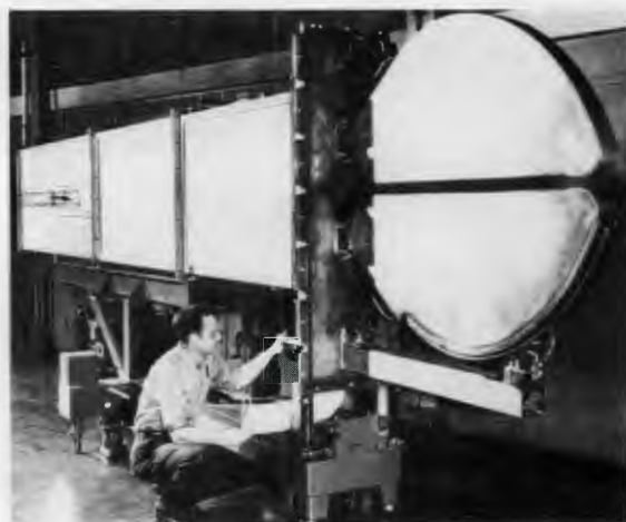
Inspection in 1952 of the 63-inch cyclotron dees.
