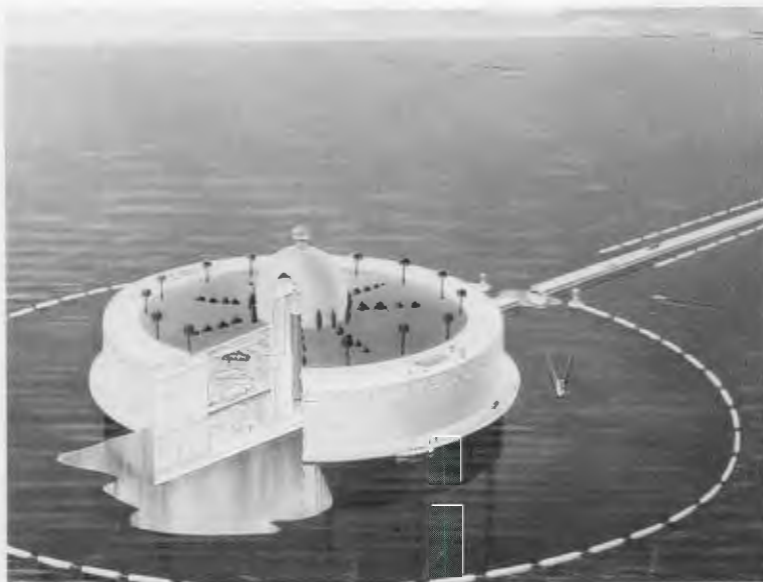
Artist's sketch of a proposed island “nuplex” using nuclear energy to generate electricity and desalt seawater for irrigating crops.
