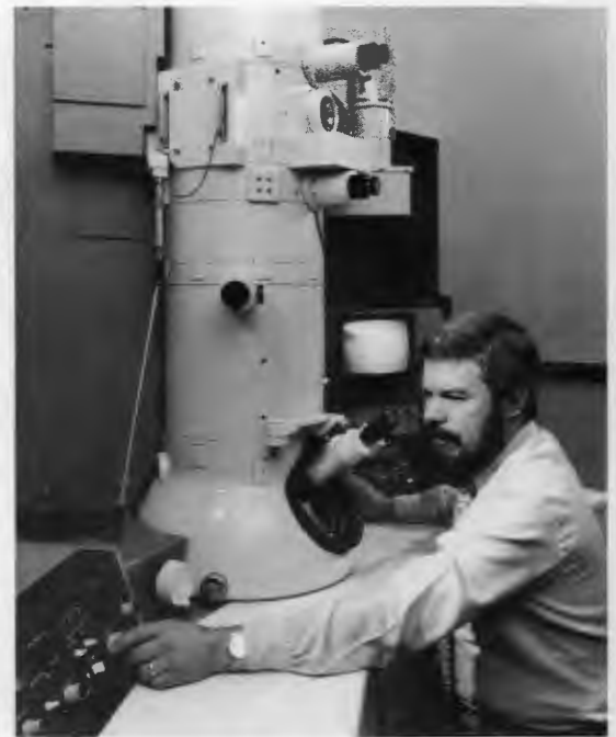
Larry Allard operates a high-resolution, transmission electron microscope to study high-temperature superconducting materials.
