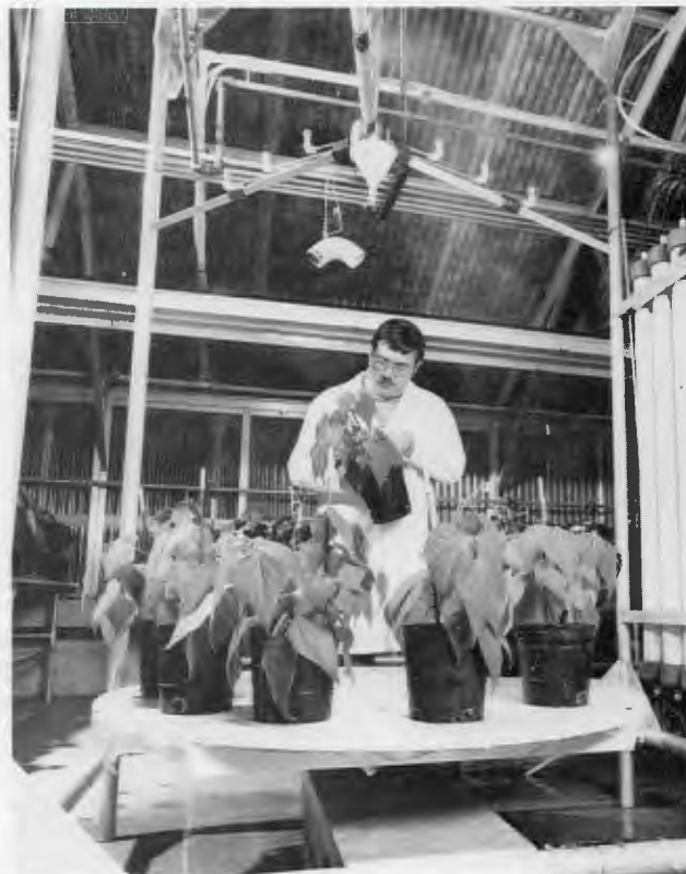
David Shriner examines bean plants in a rainfall simulator to assess the effects of acid rain on vegetation.
