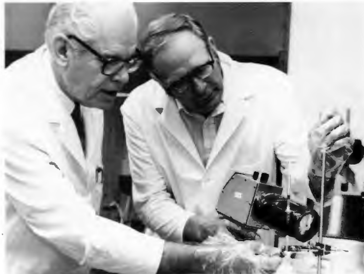
Tom Butler adjusts the ORNL-developed iridium generator used to identify infant heart defects while Clarence Guyer monitors the radioactivity with a dosimeter.
