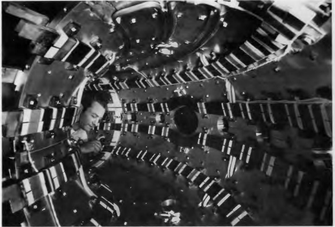
Inside ORMAK, the Laboratory's first tokamak, which achieved a plasma temperature of 20 million degrees.
