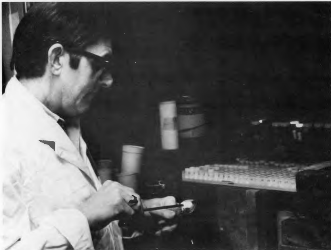
Joseph Northcutt loads coolant water from the Three Mile Island reactor after the 1979 accident. He used neutron activation analysis to determine the amount of uranium present to assess the extent of fuel melting.
