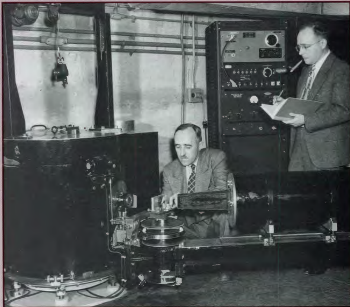
Ernest Wollan and Clifford Shull conducted some of the world's first neutron scattering experiments using this diffractometer built at ORNL and installed at the Graphite Reactor in 1950.
