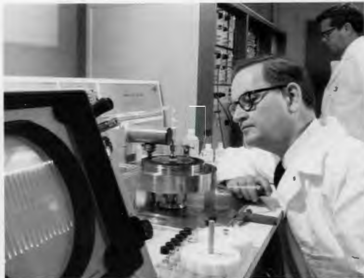
Norman Anderson and Warren Harris observe the GeMSAEC fast analyzer, a 1968 diagnostic instrument later commercialized.
