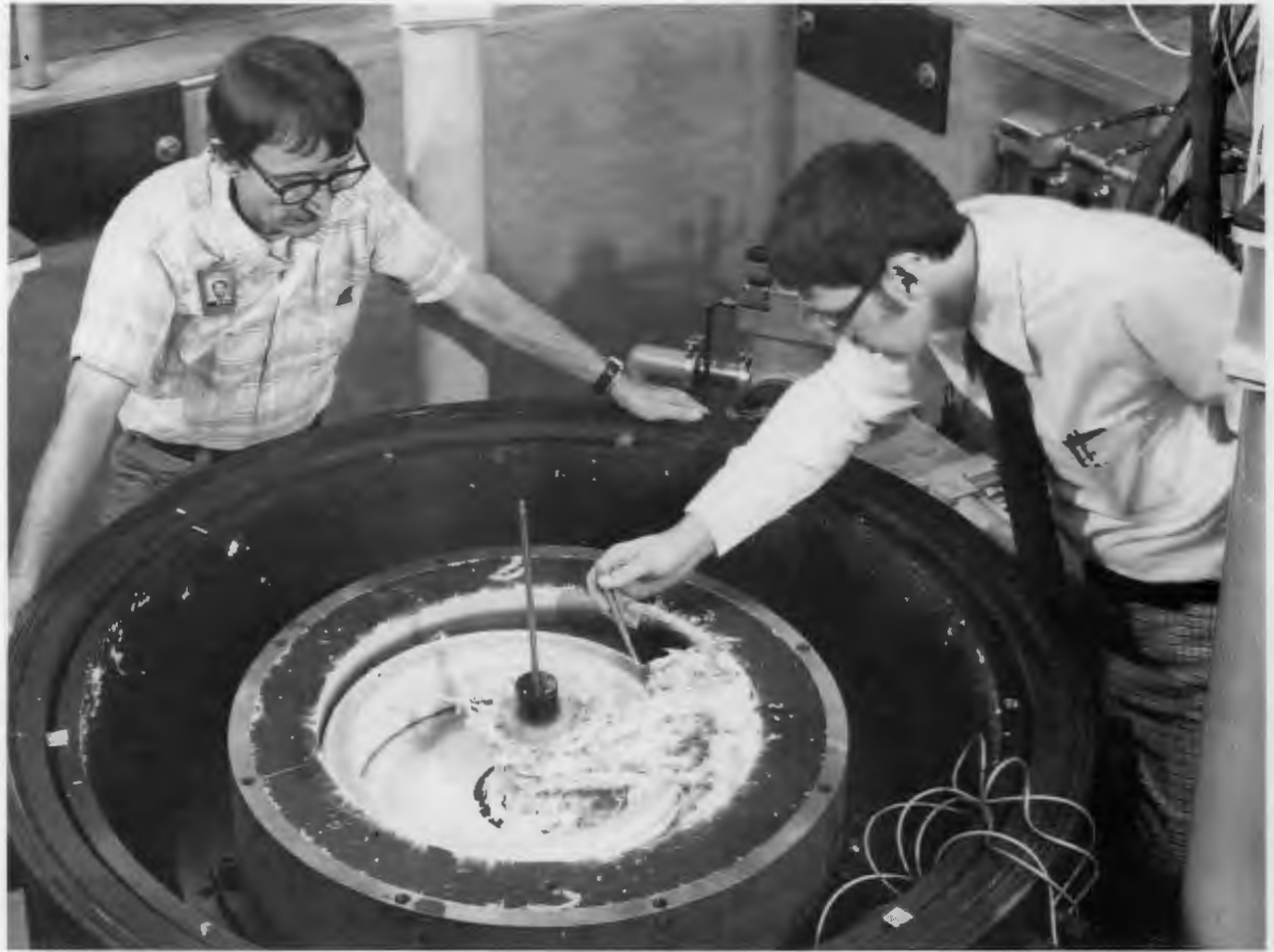
Robert Steele and B. J. Sutton evaluate materials in a 1980 flywheel under study for mechanical energy storage in automobiles. Flywheels were also explored as energy storage devices for the Strategic Defense Initiative.
