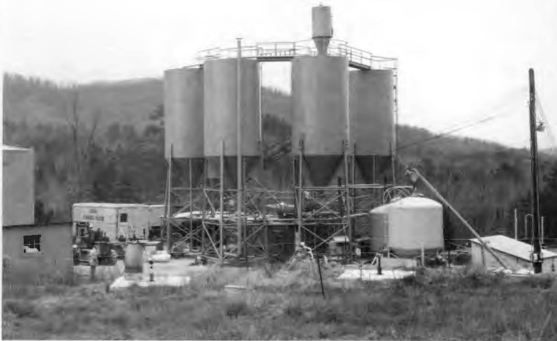
One of the Laboratory's hydrofracture facilities that injected wastes into subsurface strata.
