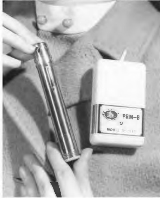
Personnel radiation dosimeters of the 1950s and 1960s included the pocket screamer, or "chirper."
