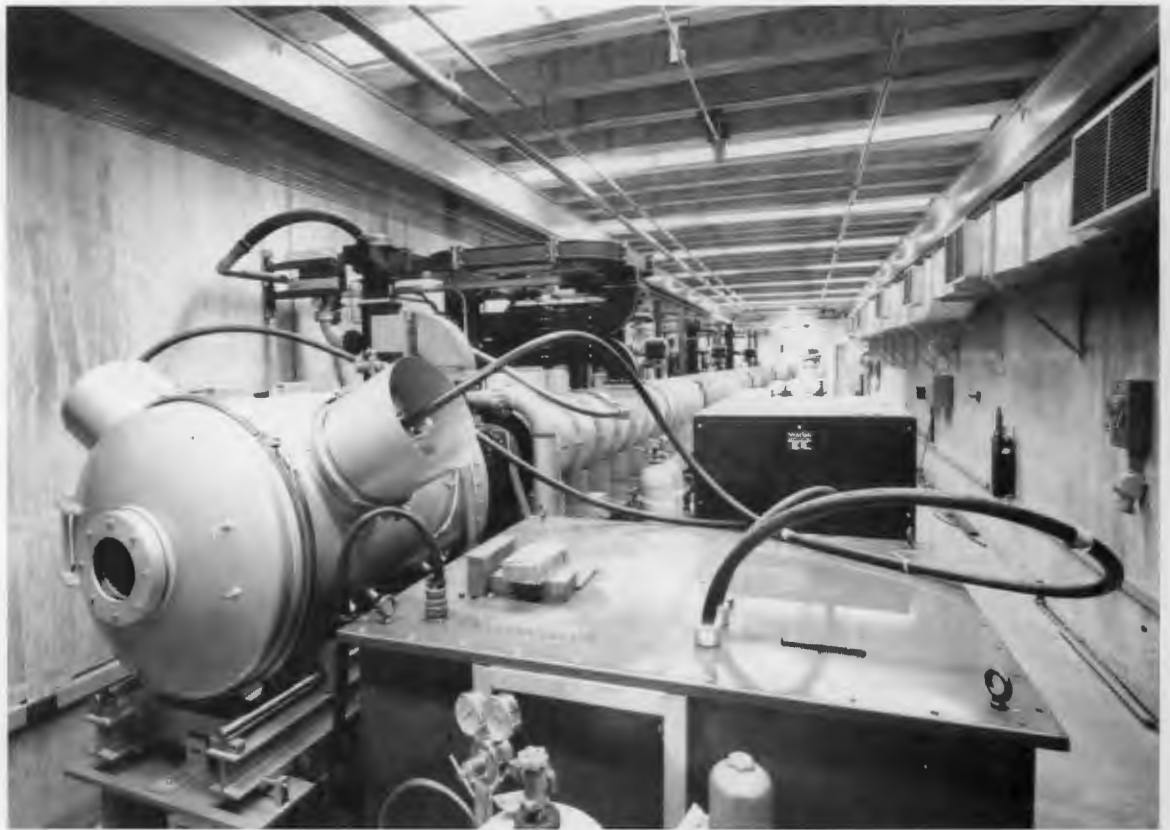
Original electron injector and linear accelerator of the Oak Ridge Electron Linear Accelerator.
