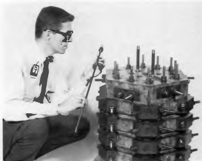
Jim Corum examines a prestressed concrete test vessel for an experimental gas-cooled reactor.
