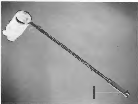
The Laboratory helped develop scoops used by Apollo astronauts to retrieve lunar rocks and soil samples.
