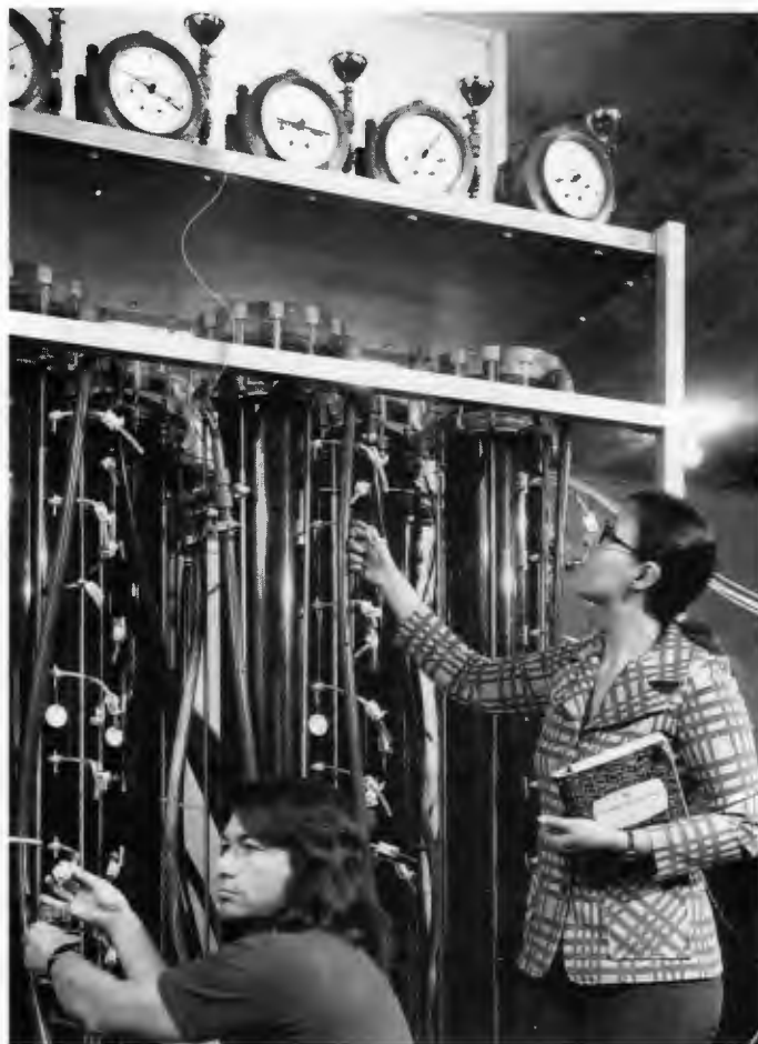
Bill Griffith and Alicia Compere examine the anaerobic biological reactor called ANFLOW, tested at the Laboratory during the 1970s.
