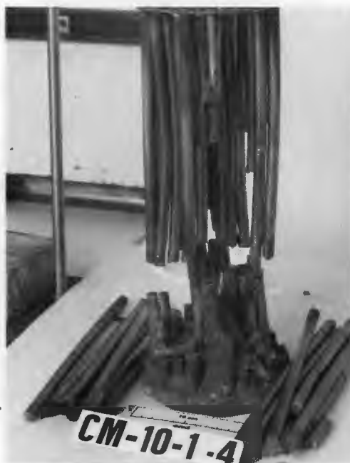
Nuclear safety experiments at the Laboratory during the 1970s and 1980s included heating bundles of reactor core rods until they melted.
