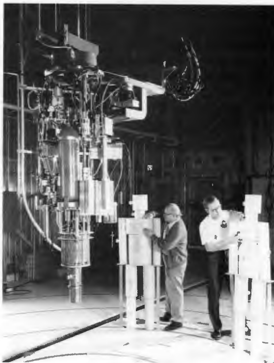
Phantoms for estimating radiation doses in the human body are checked at the Health Physics Research Reactor.
