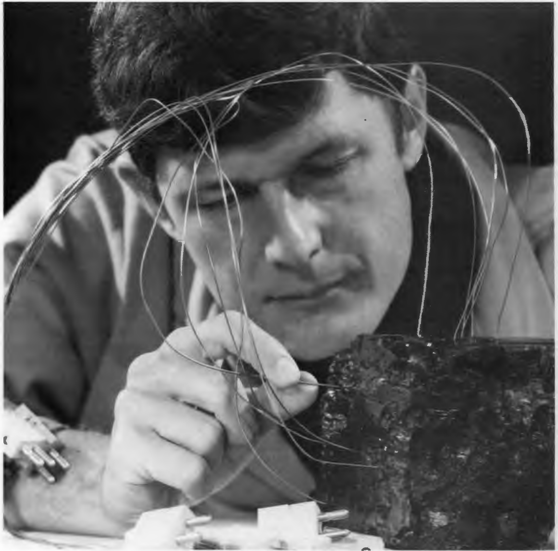
Richard Forrester measures heat transfer in coal blocks for coal gasification studies.
