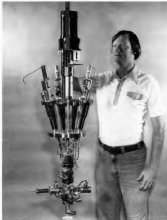
Stephen Combs adjusts a pneumatic injector developed at the Laboratory to shoot pellets of frozen deuterium into the plasmas of fusion reactors.
