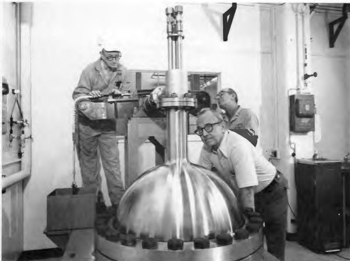
Craftsmen B. E. Burdette and W. A. Wilburn and engineer Malcolm Richardson, in foreground, adjust a nozzle-to-sphere test machine for the Liquid Metal Fast Breeder Reactor Program in 1975.
