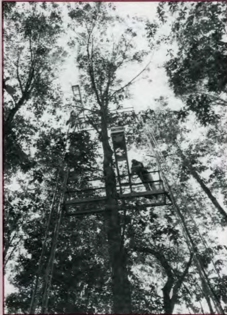
Environmental scientists use treetop samplers to study the transport of airborne materials to forests and their soil.
