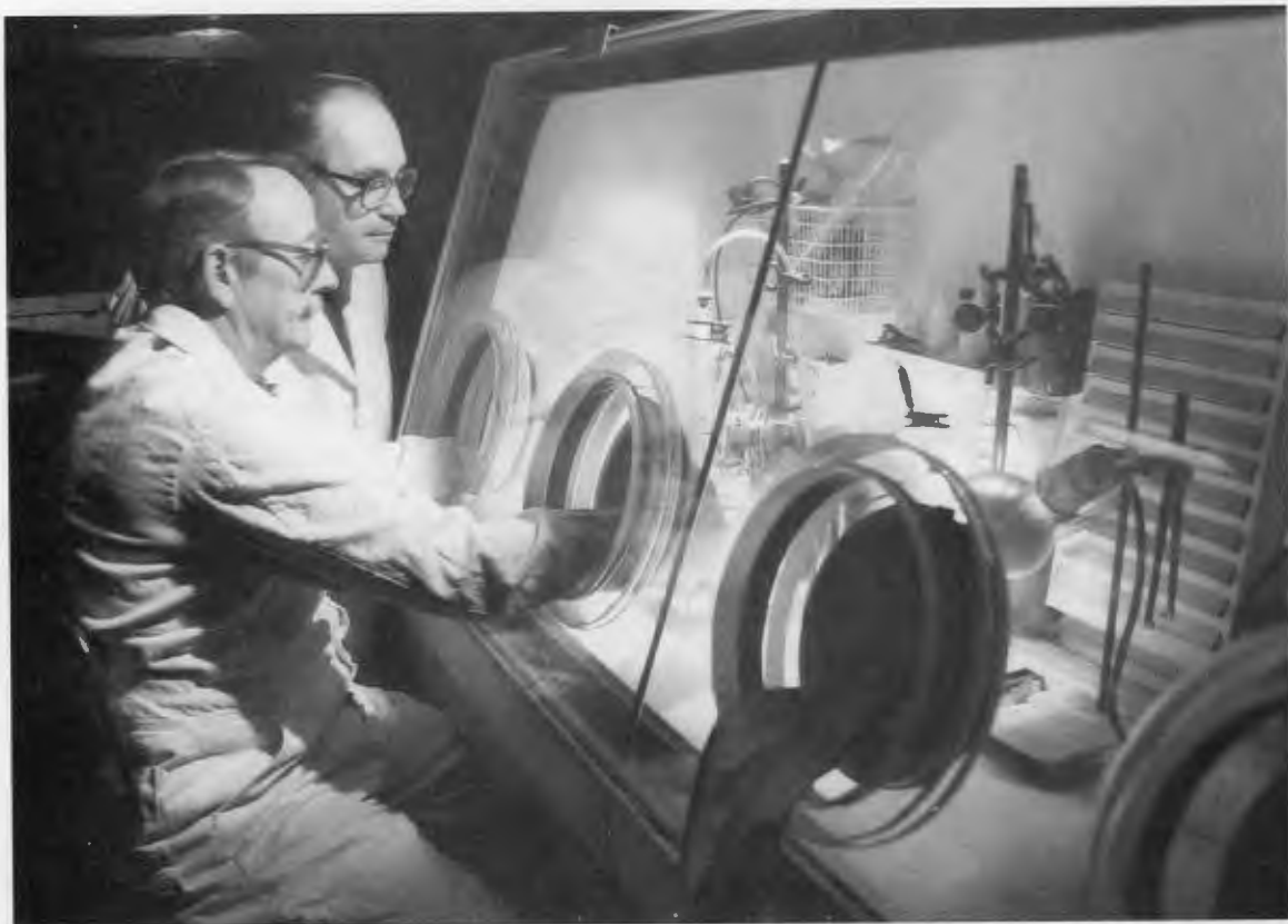
Lew Keller watches as Chick Wiggins uses a protective glove box at the Transuranic Processing Plant to achieve final purification of the transplutonium elements produced in the High Flux Isotope Reactor.
