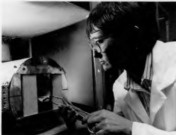
Claudette McKamey inserts a corrosion-resistant iron aluminide specimen into a furnace to test its strength and ductility.
