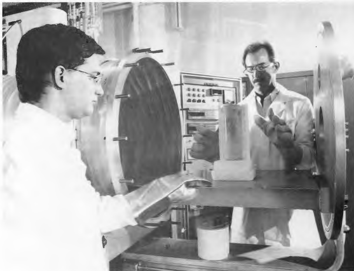
Hal Kimrey and Mark Janney inspect a silicon carbide ceramic tube that has been heated by microwaves.
