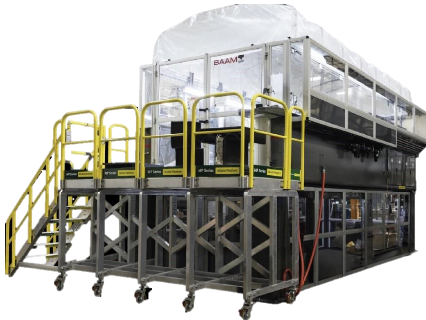
Figure 10. Cincinnati BAAM Used to print the composite AM Nodes and Casting Patterns
