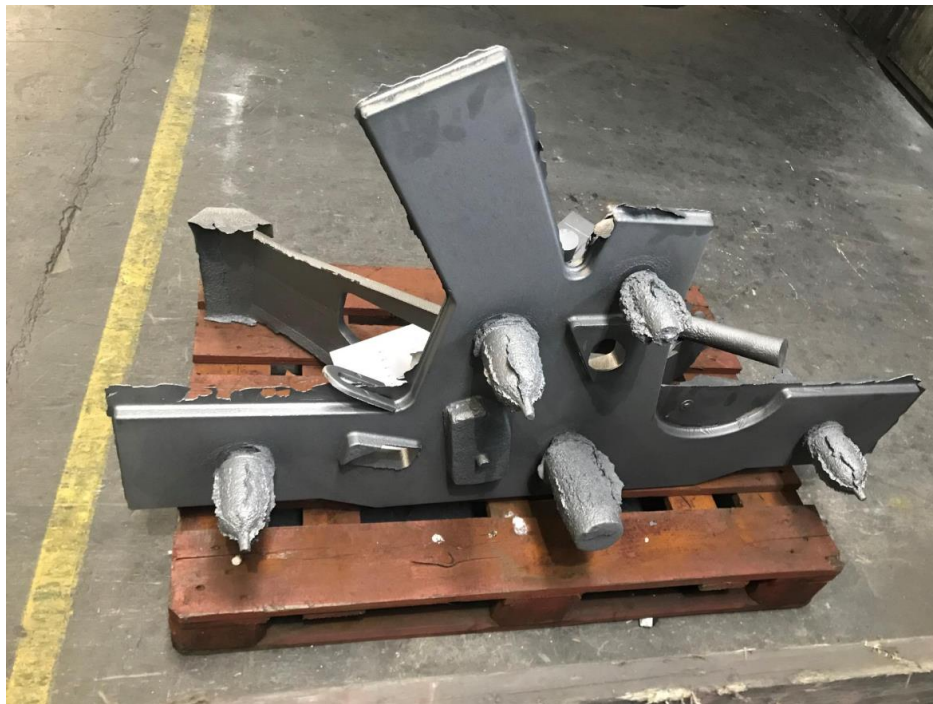
Figure 37. Cast SN with risers and runners still attached
