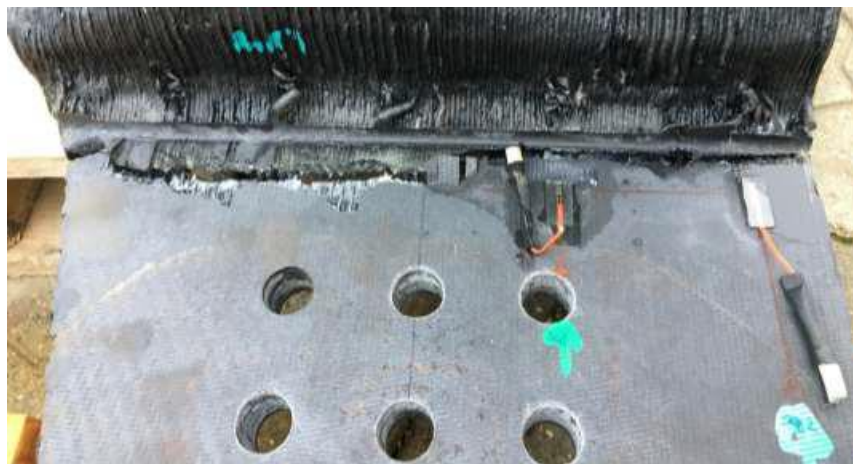
Figure 47. Composite V2 node failure Arm 5
