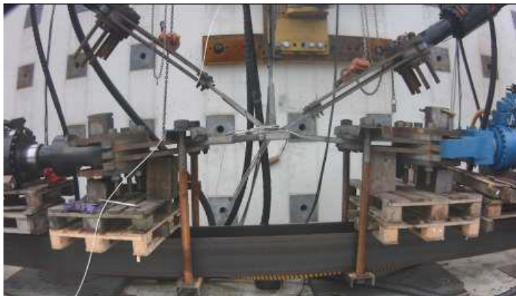
Figure 50. A cast node during testing
