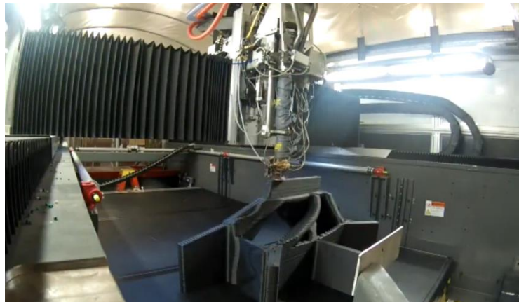
Figure 18. Printing the V1 Composite structural node
