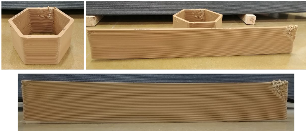
Figure 7. Printed hexagon and a curl bar showing the print quality and slight warpage at the edges.
