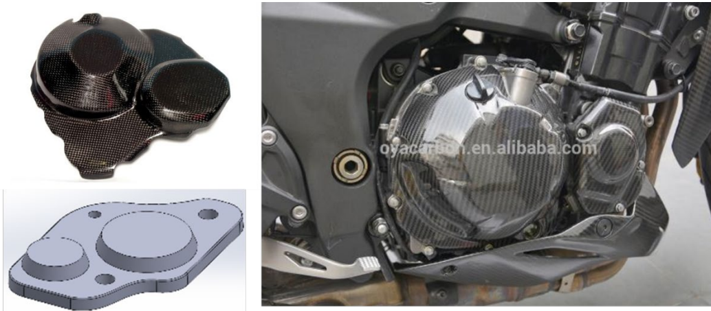
Figure 8. Motorcycle cover as selected demonstration mold: Actual part and a selected CAD design.
