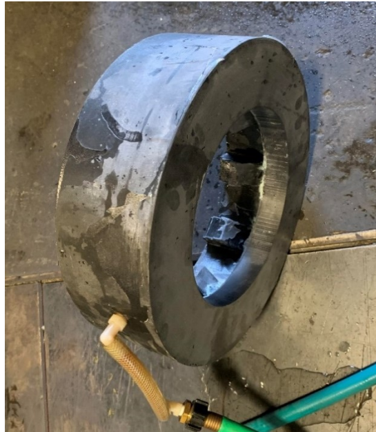
Figure 8. Infused and Machined Stator Outer Housing
