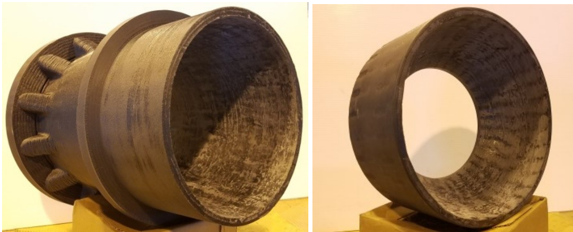
Figure 3. Printed Draft Tube (L) and Bell Plug (R)
