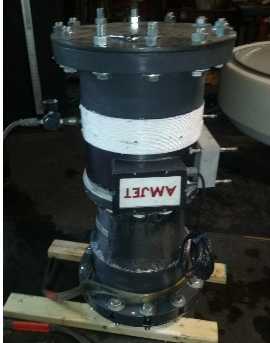
Figure 5. Assembled Unit for Pressure Test
