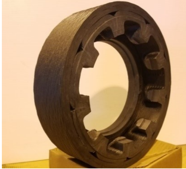
Figure 4. Printed Stator Outer Housing
