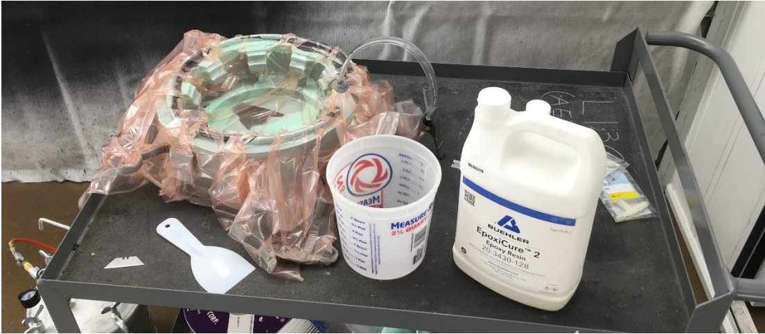
Figure 7. Vacuum Infusing Resin
