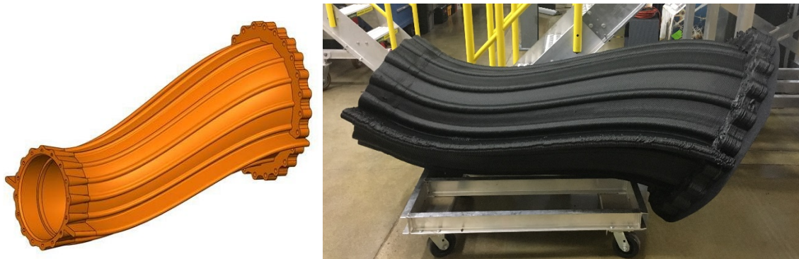
Fig. 6. The CAD model of the thimble (left) and the final printed version (right).
