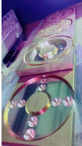
Fig. 9. Runner spacer plates provided by Cadens
