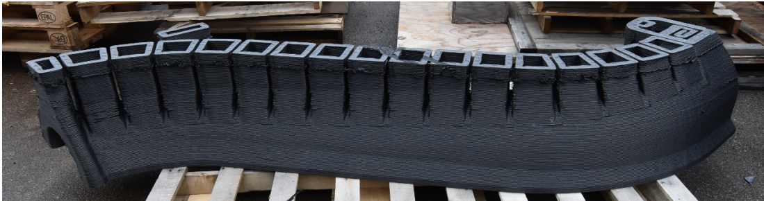
Fig. 4. The first half of the draft tube as printed. It is flipped upside down, so the support structures are seen on top.
