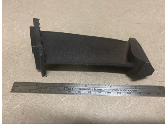
Figure 9: EBM Inconel 738 airfoil fabricated defect-free after geometry and process optimization.
