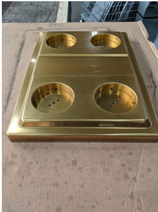
Figure 4. Printed Whirlpool die after machining and nitriding.
