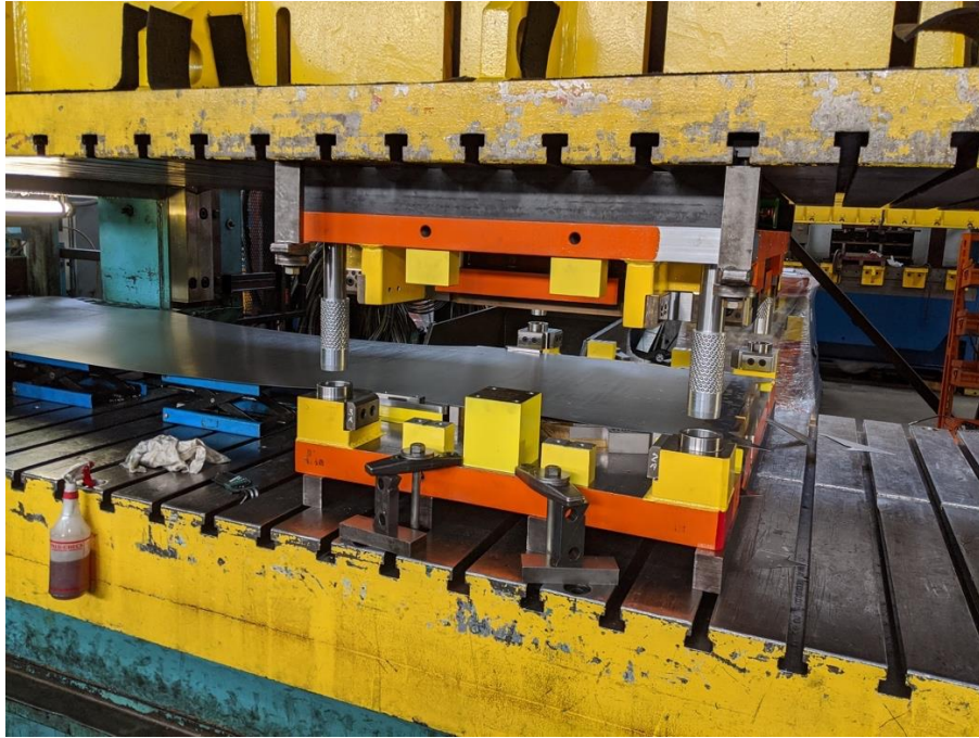
Figure 5. Chelar Industries stamping press used for demonstration.
