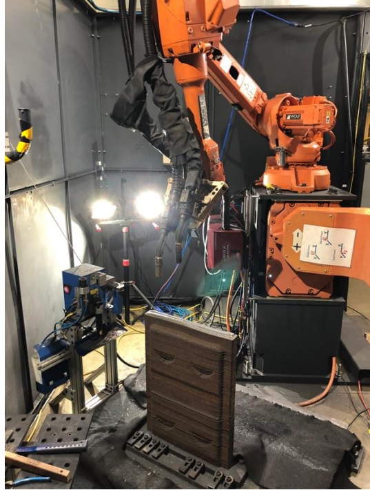
Figure 3. Whirlpool die at print completion.
