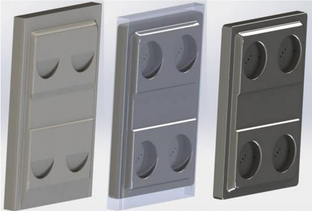
Figure 1. As-printed CAD, as-printed overlaid on as machined CAD, and as-machined part CAD.
