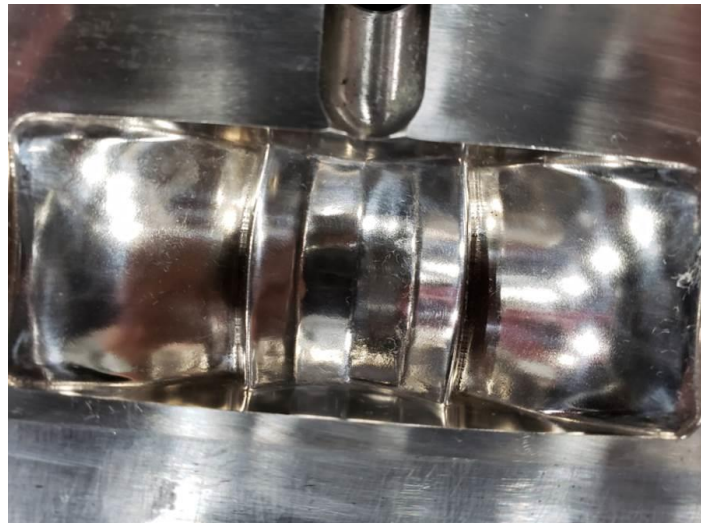
Figure 7. Mold surface after polishing.
