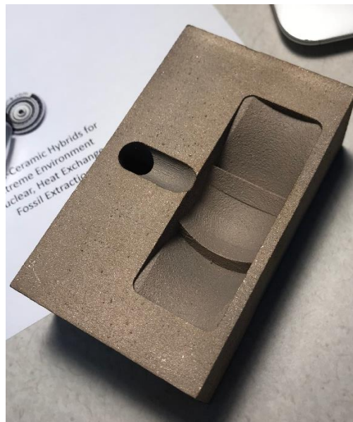
Figure 6. One half of the fabricated mold prior to polishing.
