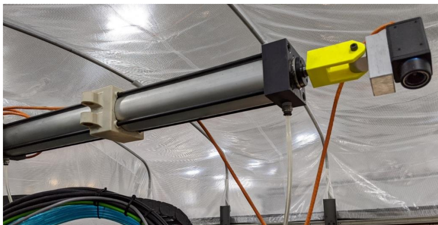
Figure 2. BAAM IR camera at the end of a pneumatic arm for extending/retracting
