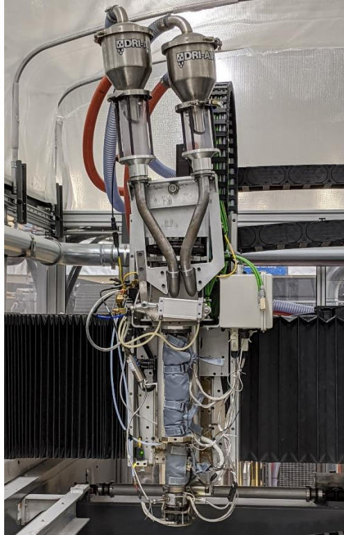
Figure 11. Multi-material system installed on BAAM. Note the two silver hoppers that house and feed the extender two different materials
