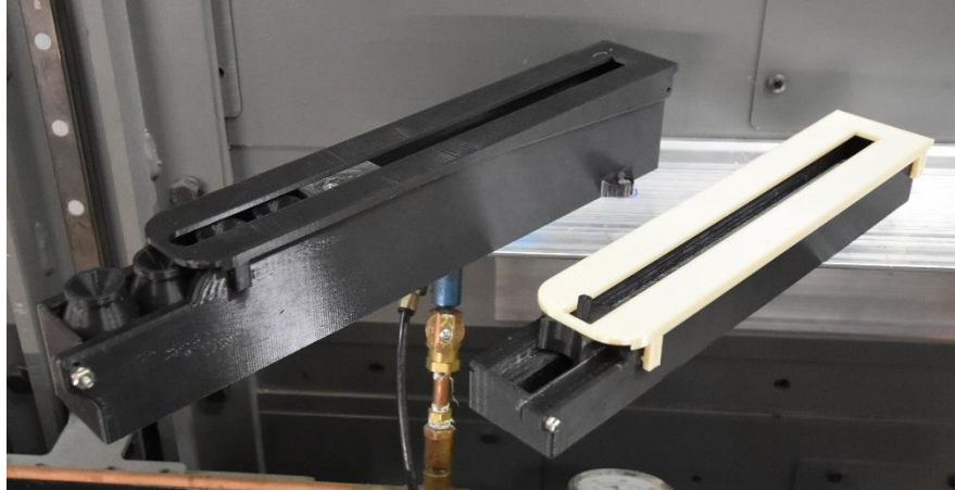
Figure 9. Magazine for holding sensors on the left and magazine for holding tracker pucks on the right
