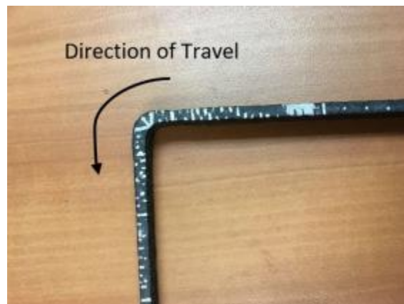
Figure 6. Printing a 90° corner with the system ID model
