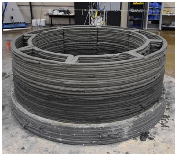
Figure 3. Test article with geometry similar to wind turbine pedestal
