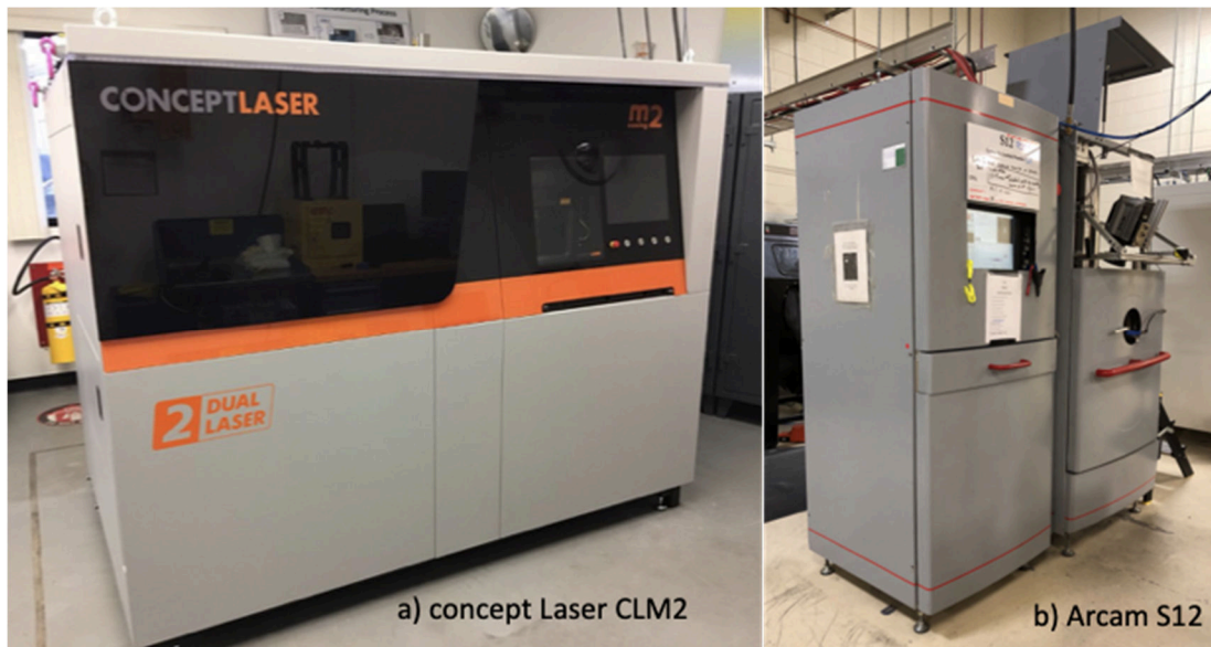
Figure 2: a) LB-PBF Concept Laser M2 machine, b) EB-PBF Arcam S12 machine
