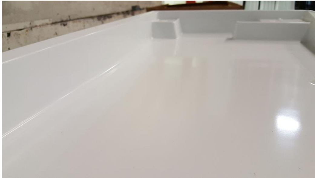
Figure 3. Manufactured Freezer Door from AM Tool
