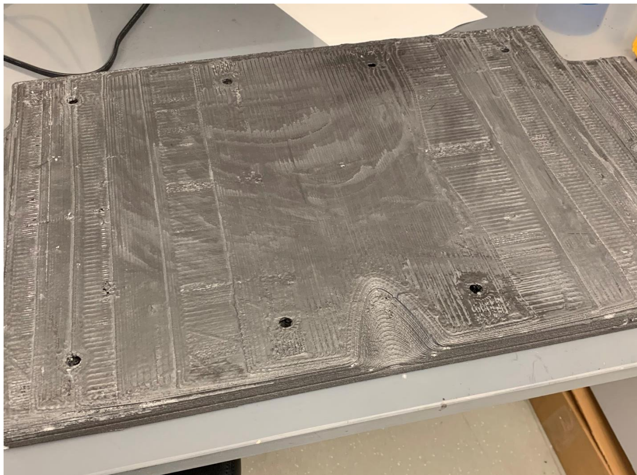
Figure 15. Mid-scale Printed High Thermal Conductivity Tool for Amana Refrigerator Door
