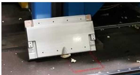
Figure 1. Production Freezer Door Foaming Mold
