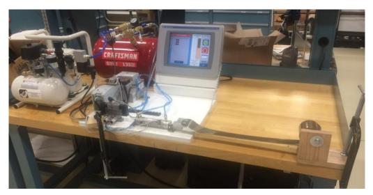
Fig. 6. Load testing with constant force springs.
