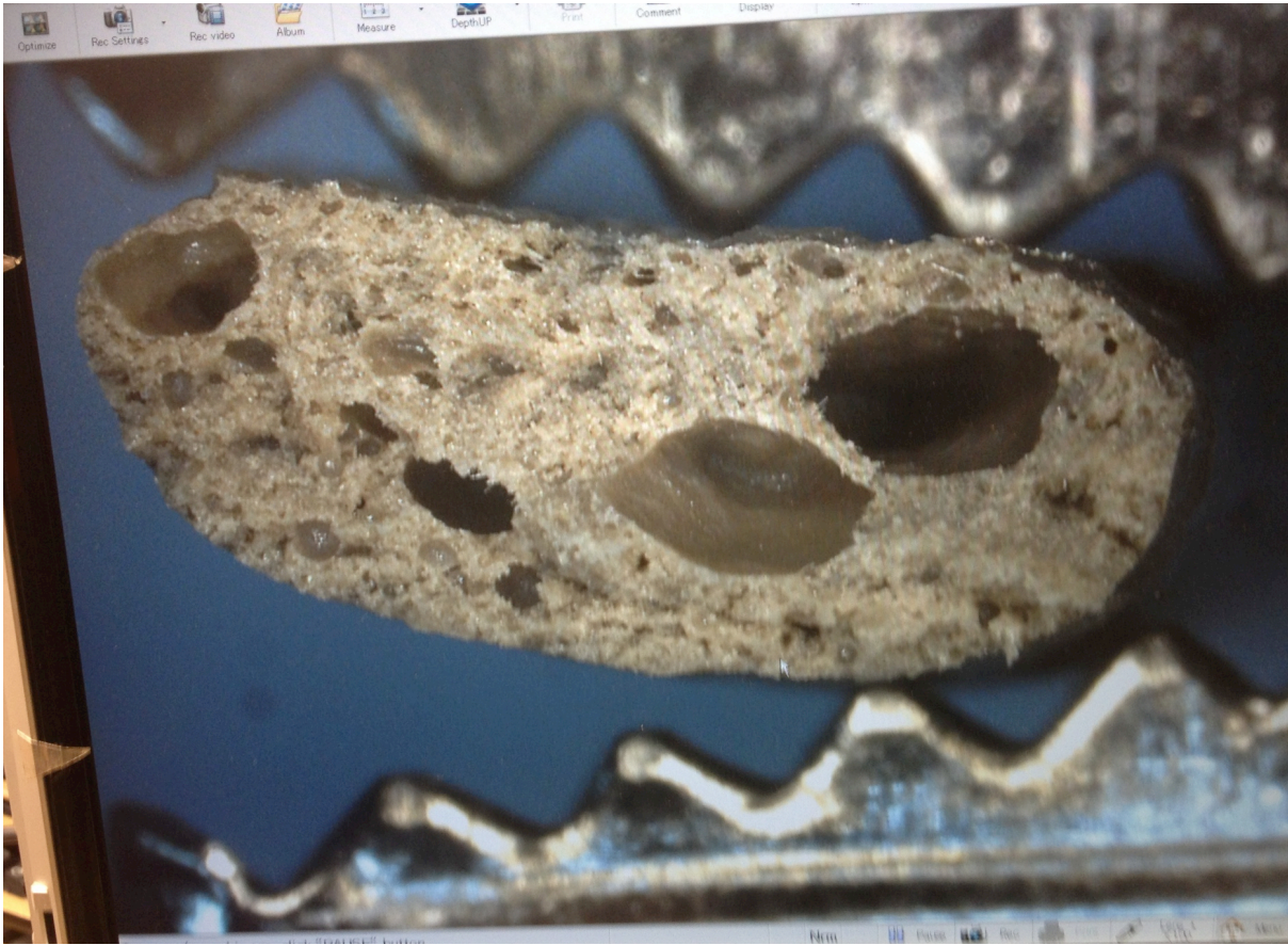
Figure 6. Cross section of GF-PPS deposited bead demonstrating significant porosity.
