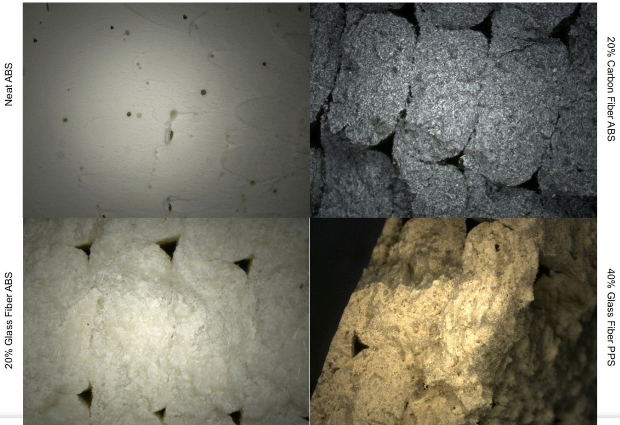
Figure 7. Fracture surface of BAAM deposited materials: neat ABS (upper left), CF-ABS (upper right), GF-ABS (lower left), GF-PPS (lower right).
