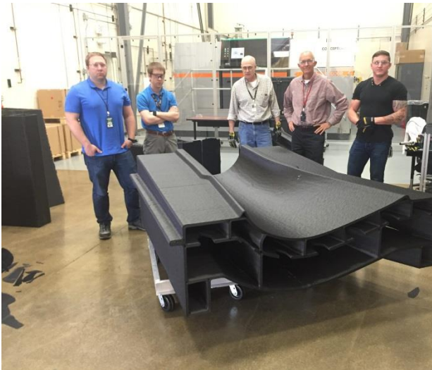
Figure 9: Section of wind turbine mold.
