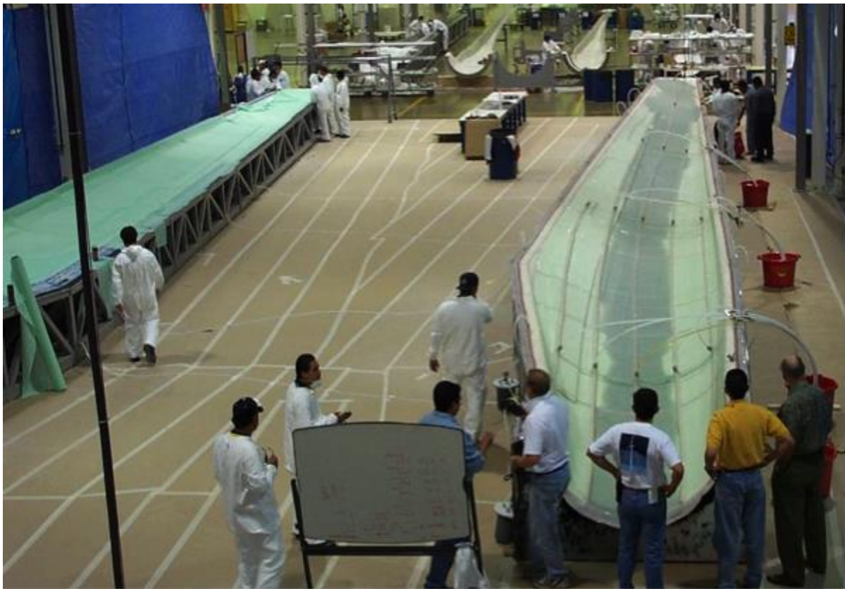
Figure 5: Resin infusion on wind turbine molds.
