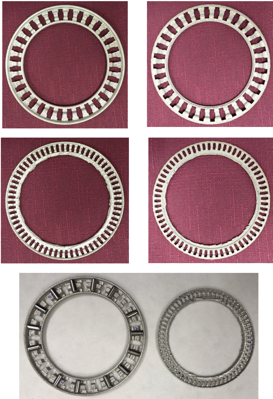
Fig. 3. Cages printed on the Renishaw out of 316L stainless steel. Large cage above (top and bottom surface). Small cage in the middle (top and bottom surfaces). Top of both large and small cages below.
