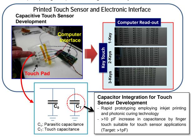
The ultimate goal of 2D and 3D additive printing technologies is to fully print electronic components and systems. An all-printed electronic circuit was developed to demonstrate the potential of innovative photonic curing technique and additive digital printing to meet the demands of high volume and low-cost roll-to-roll manufacturing technology.
