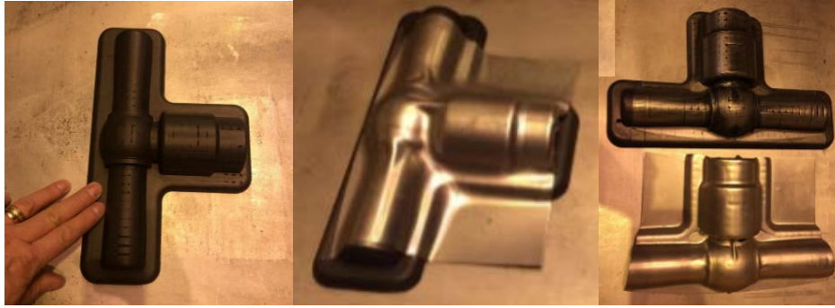
Figure 15. The male additively manufactured tool (left), tested with a 1mm blank at 30 MPa (center), and at 80 MPa (right).
