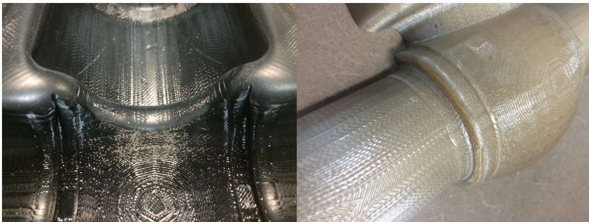
Figure 10: Female ABS die (left), and male ULTEM die (right), both exhibiting minimal deformation after repeated use at higher pressures.
