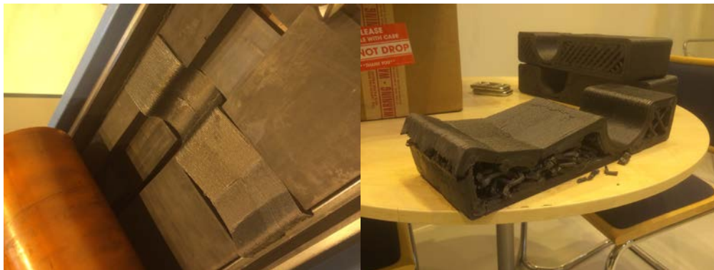
Figure 5: Failure of the low fill density specimen at 4 MPa.
