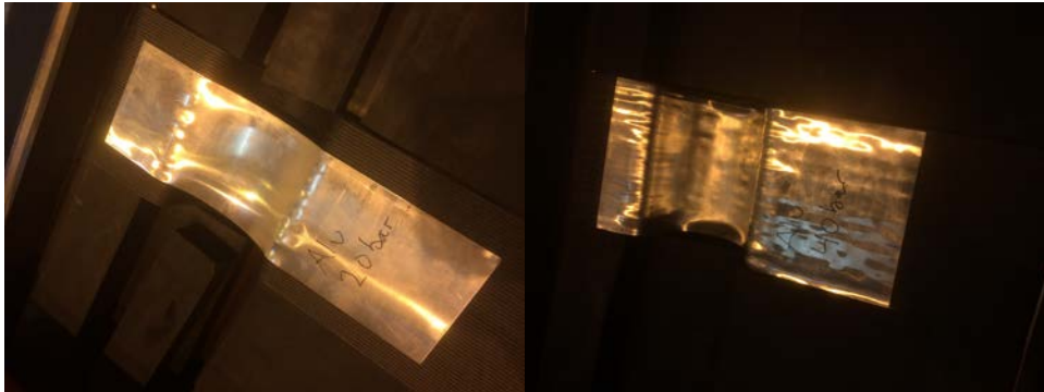
Figure 4: The low fill density tool tested at 2MPa (left) and 4 MPa (right) using Al 1050 sheet.
