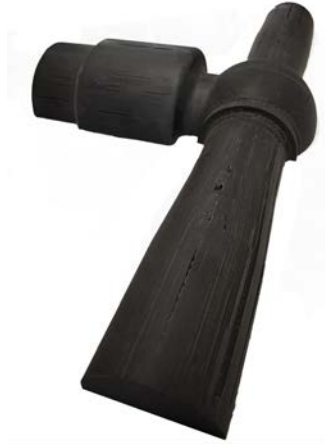
Figure 3: 8-inch diameter valve internal tool at 30% above scale.
