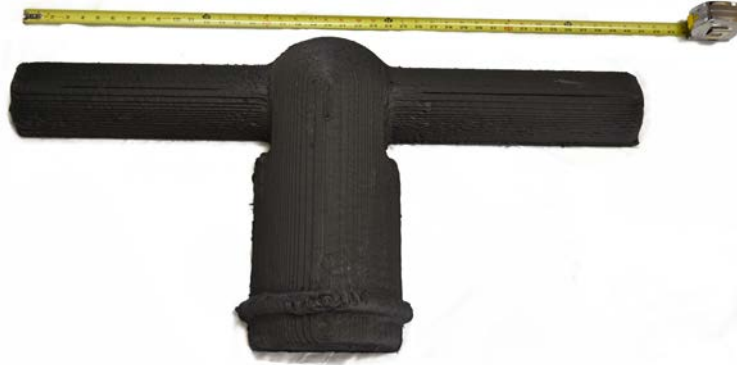
Figure 2: True scale 8-inch diameter valve internal tool.
