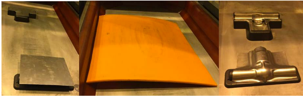
Figure 12. Female and male PPS+50% CF tools with blanks (left), placement of the rubber mat (center), and final results (right).
