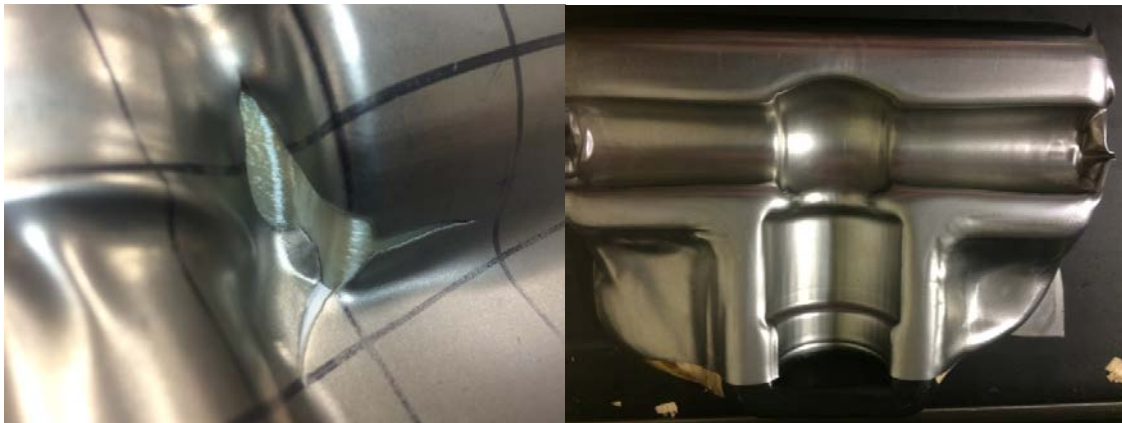
Figure 8: Failed (left) and successful (right) hydroformed net shapes.
