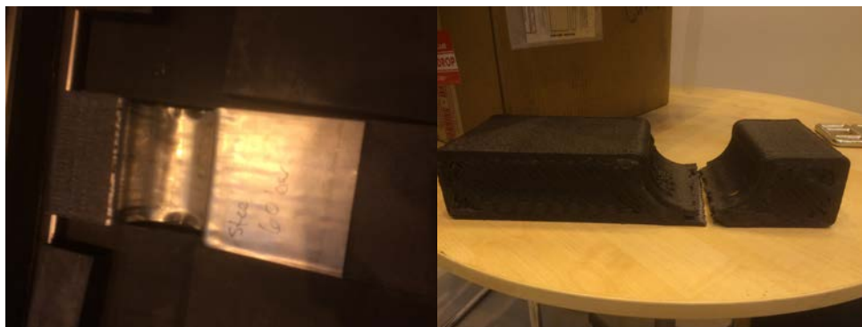
Figure 6: High fill density specimen tested at 6 MPa testing steel sheet (left) with the resulting failure of the specimen (right)
