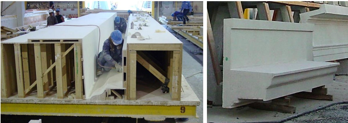
Figure 3. Left: Molds for precast concrete are typically manually assembled with sheets of plywood that are surfaced with fiberglass-reinforced coatings. Right: Precast concrete piece used as part of a building facade.
