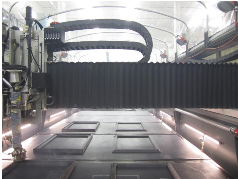
Fig. 1. Window frames shown during the additive manufacturing process.
