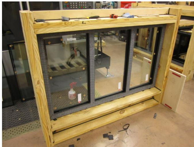
Fig. 6. Three AM window frames inserted into constructed frame.
