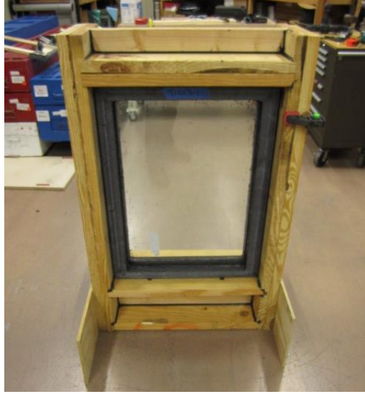
Fig. 7. A single AM window frame inserted into constructed frame.
