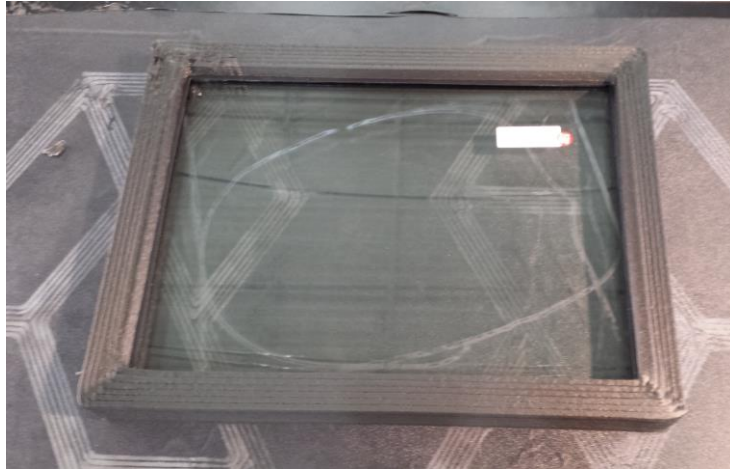
Fig. 5. AM window frame with glass inserted.
