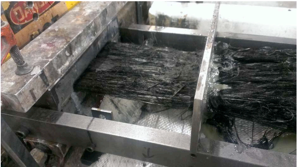
Fig. 2. Example problems with getting the Kaltex-based large tow through the pultrusion process.
