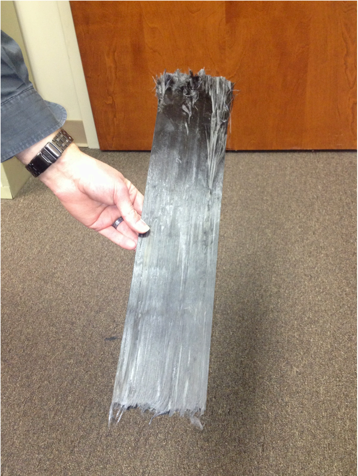
Fig. 3. Best pultruded composite section produced from Kaltex-based large-tow fiber.
