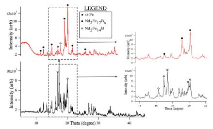
**Fig. 3.** XRD patterns obtained from the powder (shown below in black) and the build (shown above in red). Note the sharp decrease in the intensity of the peaks corresponding to the  $Nd_2Fe_{14}B$  hard magnetic phase in the additively manufactured samples. Also note the corresponding increase in the intensity in the alpha iron peak after laser processing [10].
