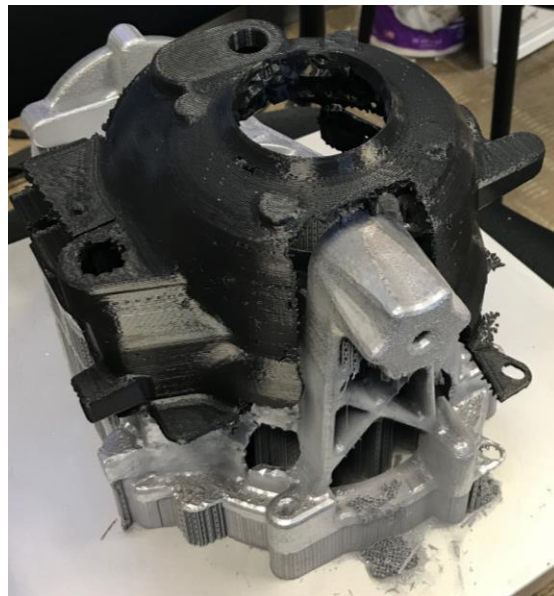
Figure 4: Assembled hybrid multi-material endoskeleton overmolded transmission housing design.
