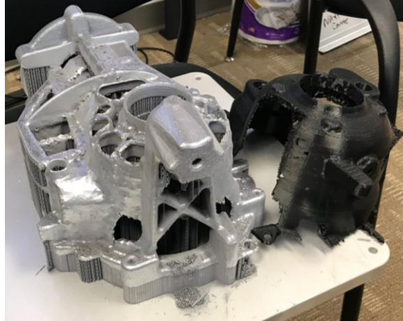
Figure 3: Prototype part manufactured using a Concept Laser laser powder bed system.
